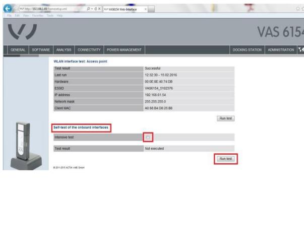
14. The screen should show the test as 'Successful'. If you see 'Failed' within the field, remove your VCI head and separate from the Wifi attachment, then reattach and place back into the Docking station and retry
